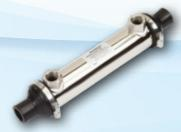
The DC is a compact, efficient single pass oil cooler suitable for engines up to 180kW, with durable cupro-nickel tubes and a choice of neoprene seawater connections. Models are also available for fuel cooling.
