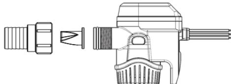
Periodically remove, clean and inspect bilge pump, check valve and its surroundings for damage or debris that may reduce the performance of the pump.
