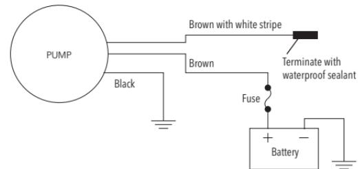
**On 12 volt pump:** Minimum voltage of 10.5 volts required.
